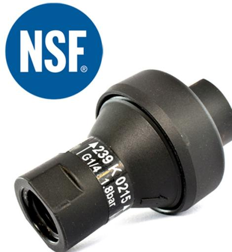
The pre-set EcoReg® fluid regulator is an independent diaphragm pressure regulator that can be installed in all fluid systems. The pressure regulator ensures a constant and precise output pressure independent from the input pressure. The pressure value has been factory preset and cannot be changed. This ensures that no one can manipulate the specified pressure value.
